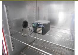
High Temperature/ Humidity Test Low Temperature Test
